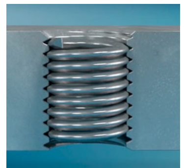
HELICOIL® Tangfree correctly installed ( 0.25 - 0.5 \times P below the surface)
